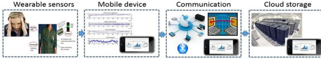
Figure 4.1: Hardware architecture of a context-aware mobile system.
